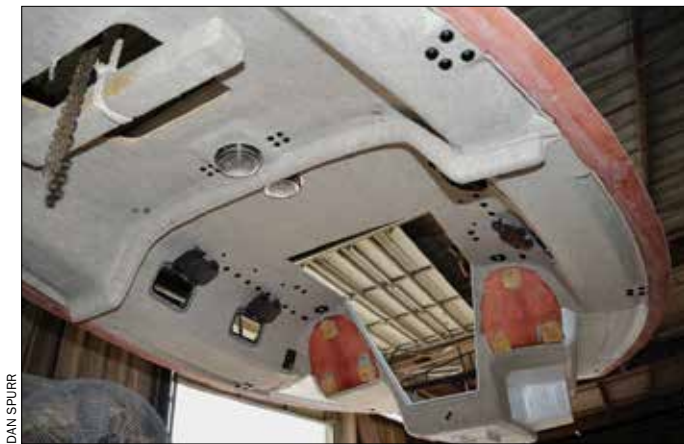
Above —A prewired deck is suspended by overhead chain hoist before it is lowered onto the hull. Right —A shop crew member with a buffing wheel details a hull before moving the boat outside and onto a trailer for delivery.
