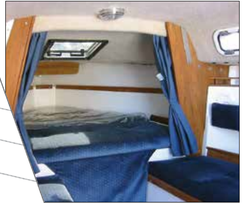
Above —Interior of the Precision 23 reveals the emphasis on economy and ease of assembly: liner with berth flats and hull sides, bulkheads fitted to liner and bolted to deck beam, and fabric overhead.
