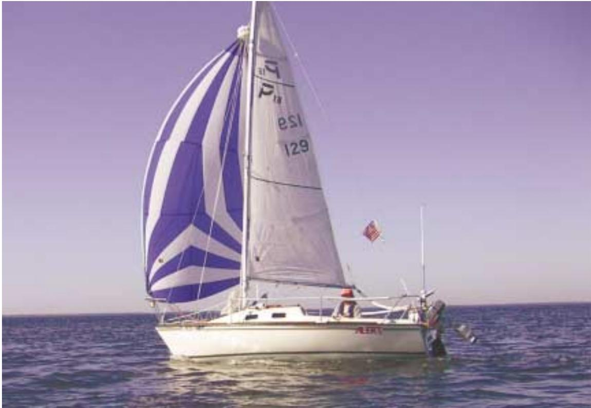
Spinnaker hardware installation was fairly simple. The halyard was mounted 14" above the jib stay attachment point to allow for a slightly larger sail, and to keep the dousing sock from wearing, or possibly snagging, there.
