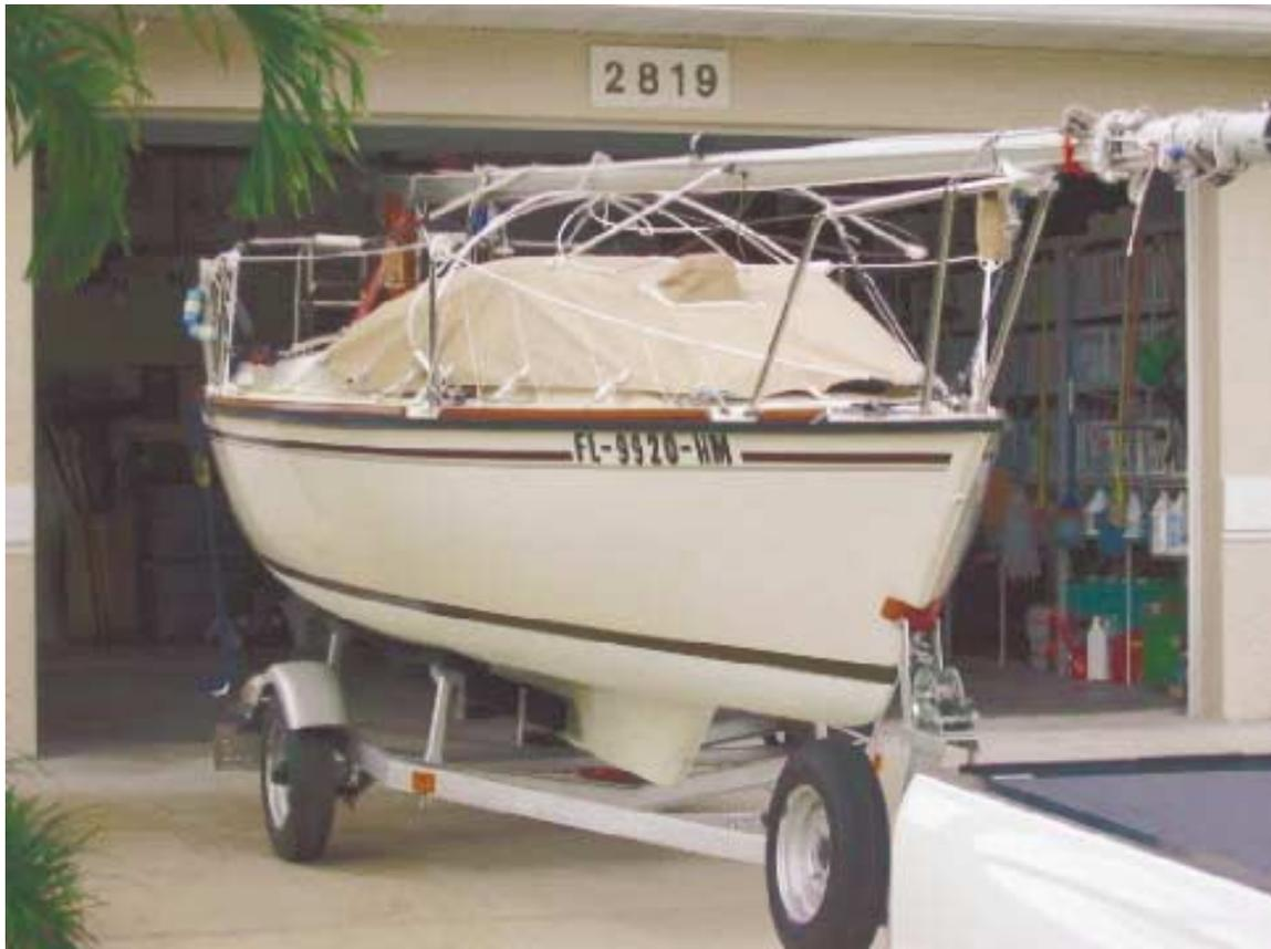
Note: When trailering the boat along the highway, I make an effort to keep my speed around 60 MPH. With some vehicles, it's possible to almost forget that this small boat is even "back there" – yet the nearly 2,000lb load is not insignificant when the time comes to stop. Keeping the speed down is probably the single best step you can take to insure that you *and* your boat arrive at your destination safely.
