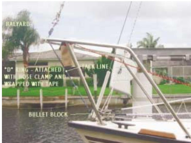
The sheets are led aft to Harken rail mounted Bullet blocks and Harken 150 Cam Cleats mounted on the beveled edge of the cockpit seats.
